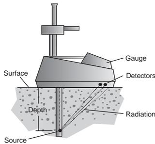
*On the right, the neutron source remains above the surface, and radiation is emitted into the ground and scattered back to the detector to provide a measurement of the moisture content.*
