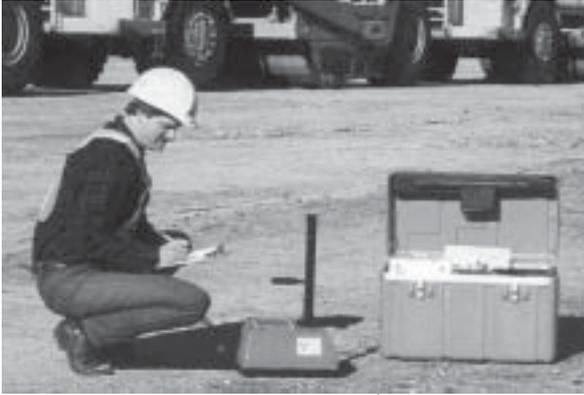
*Portable gauge used to test the structural integrity of roads and bridges*
