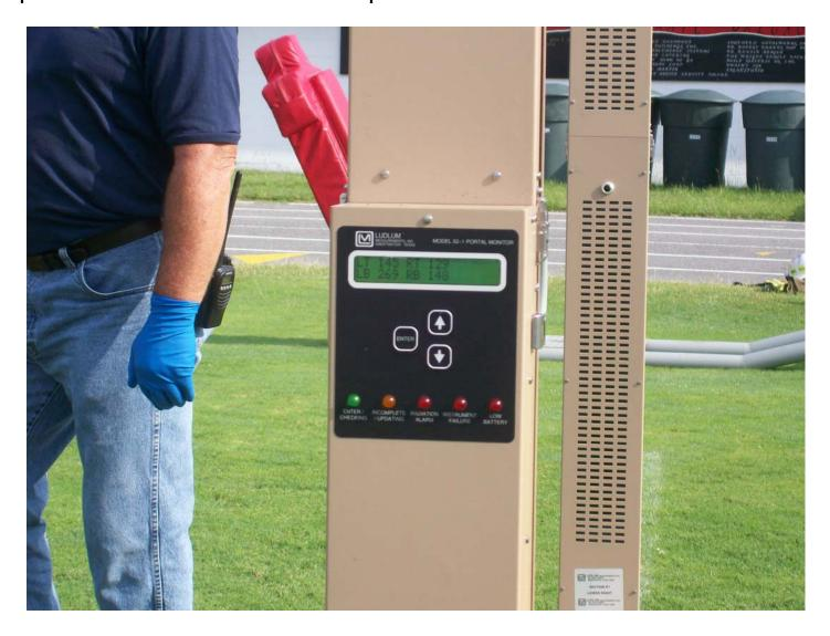
Portal Monitor should be set up so that normal vehicle can pass through with the sides fairly close to the monitors. For larger vehicles the detectors can be slid further out.
