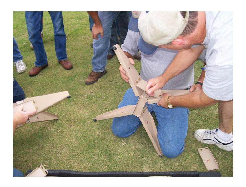
Detector panels are assembled onto the legs and a cable is ran along the ground between the panels.
