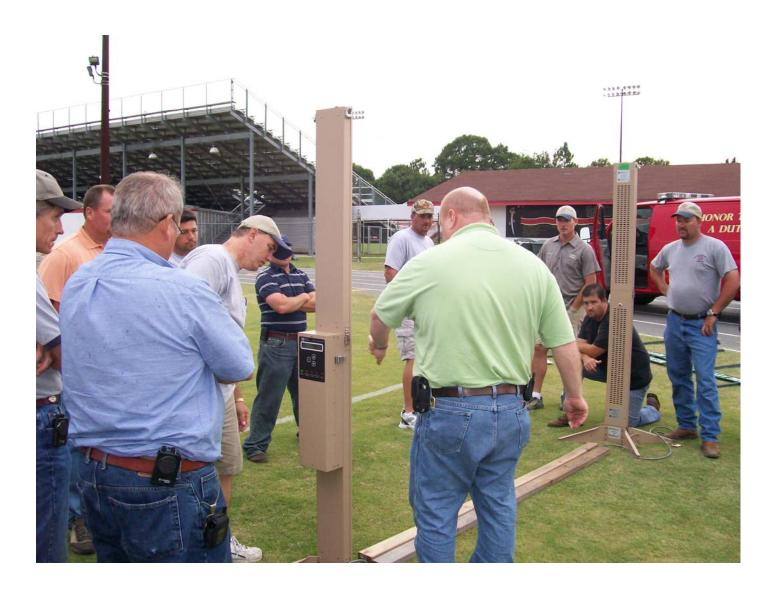
When the portal monitor is powered up the unit will go through a back ground count. All warning lights should be off and you should have a reading for all four panels when the count is complete.
